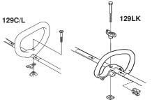
· Fit the hardware as shown in the diagram and tighten.
